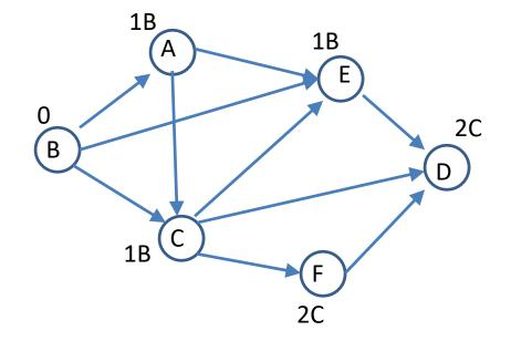
Note that we can find the path from B to any node X by walking backwards along the predecessors from X to B. This is the same way we found paths from the entrance to the exit of a maze in Lab 3. Question: Would this algorithm still work if we replaced our queue with a stack?
